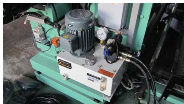
Hydraulic Actuator AO-2GH is used on a Laminator for Unwinding
