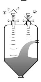
The instrument cannot be installed in the arched or domed roof intermediate. In addition to produce indirect echo is also affected by the echoes. Multiple echo can be larger than the real value of signal echo, because through the top can concentrate multiple echo. So cannot be installed in a central location.
