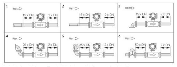
1=Reduction,2=Expansion,3=90° elbow or T-piece, 4=2x90° elbow,
