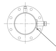
Before Welding, the base should be processed as the same as the circular arc of pipe to ensure sealing
