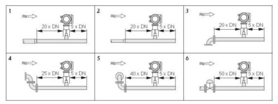
1=Reduction,2=Expansion,3=90° elbow or T-piece, 4=2x90° elbow, 5=2x90° elbow (3-dimensional), 6=Control valve or pressure regulator.
