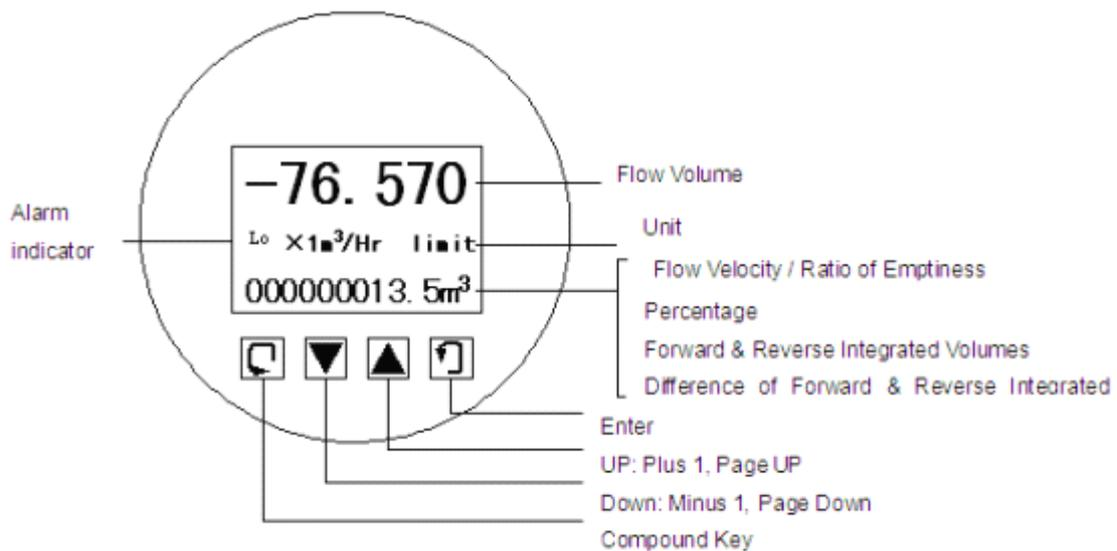
Fig.5(b) Compact-type key and display
