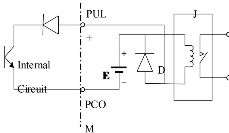
Fig.14 (f) Connection with relay (e.g. PLC)
